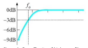
Figure 1. Cut-off point of high-pass filter
