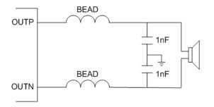
Figure 3. Typical Ferrite Chip Bead Output Filter
