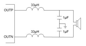
Figure 2. Typical LC Output Filter, Speaker Impedance= $8\Omega$
