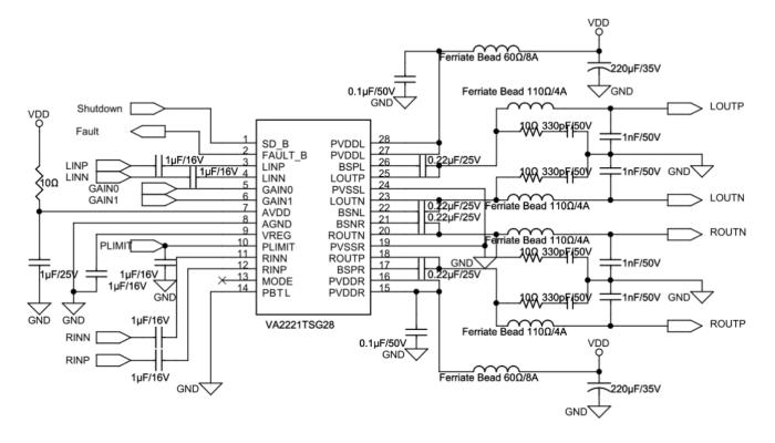
Figure 6. VA2221 Stereo Reference Application with Ferrite Bead
