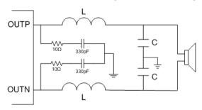
Figure 4. Output Snubber Circuits
