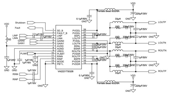
Figure 5. VA2221 Stereo Reference Application with LC Filter
