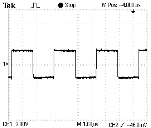
SW Noise ( V_{IN}=4.2V, I_{LOAD}=100mA )
